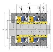
A Primary seal gas supply B Primary vent S Secondary vent
