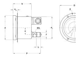
$\mathbf{D} + \mathbf{Q}$  flush mounting, front flange 4 holes; back connection.
