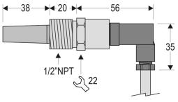
Figure 7 – Remote sensor dimensions
