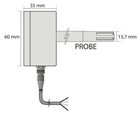
Figure 4 – Dimensions of the RHT-DM-485-LCD model
