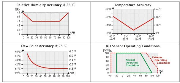
Figure 11 - Accuracy of humidity and temperature measurement
