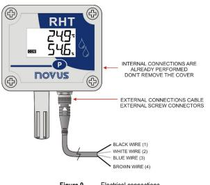
Figure 9 – Electrical connections
