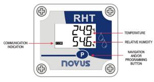
Figure 1 – Transmitter main screen
