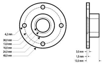
Figure 3 – Flange for fixation of the RHT-DM-485-LCD model
