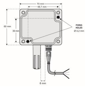
Figure 5 - Fixing bores and dimensions of the RHT-WM-485-LCD model
