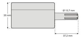
Figure 6 – Dimensions of the RHT-WM-485-LCD model
