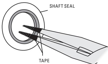
**SHAFT SEAL INSTALLATION:**
