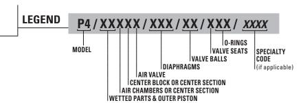
In the case where a center section is used instead of a center block, air chambers, and air valve, the designation will be as follows: Polypropylene = PPP, Acetal = LLL
