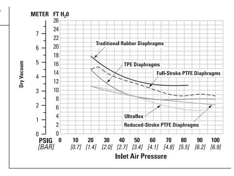
Suction-lift curves are calibrated for pumps operating at 305 m (1,000') above sea level. This chart is meant to be a guide only. There are many variables which can affect your pump's operating characteristics.
