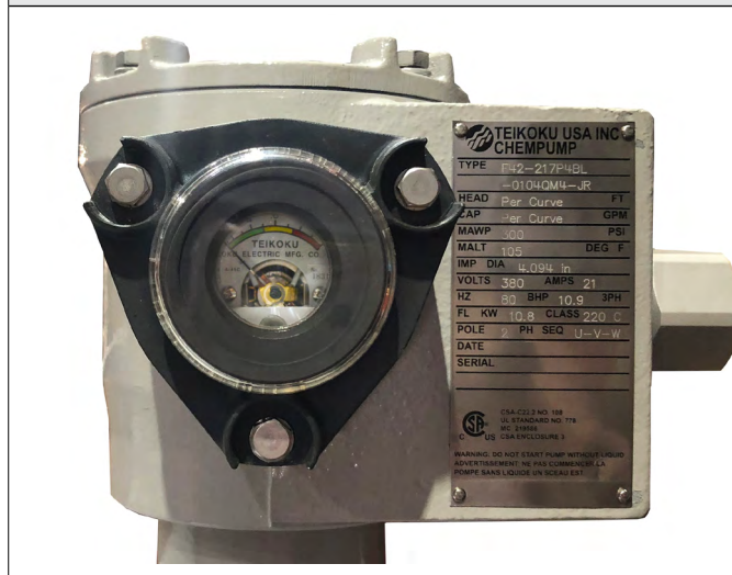
Figure 2-1. Teikoku TRG Bearing Wear Monitor
