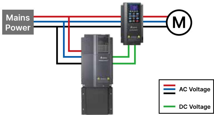
Provides the crane and hoist system four-quadrant operation and energy saving performance with the power regeneration function
