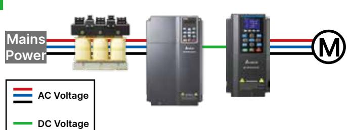
Provides the crane and hoist system excellent operation quality with reduced torque ripple, harmonic suppression, high power factors and energy saving performance with the power regeneration function
