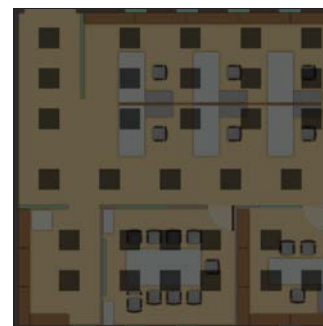
Delay time elapsed, all lights turn off.
