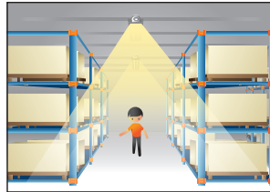
Occupancy presence Light auto on
