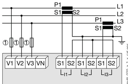
Use of 2 CTs reduces by 0.5% the accuracy of the phases, the current of which is worked out by vector calculation.
