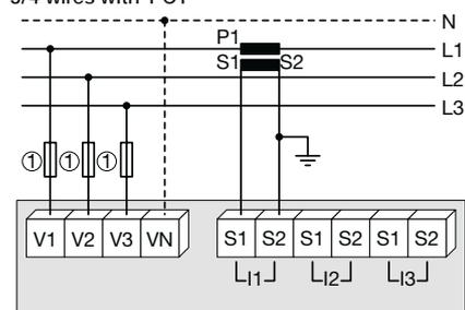
Use of 1 CT reduces by 0.5% the accuracy of the phases, the current of which is worked out by vector calculation.
