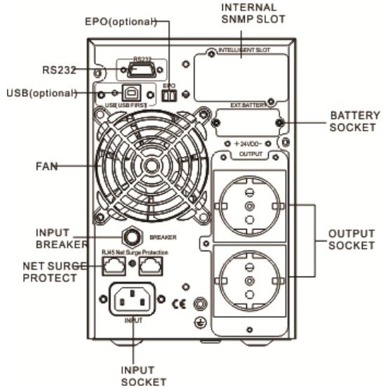
**FIG.2 1kVA Rear Panel view**
