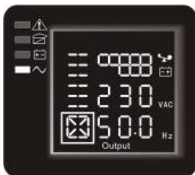
LCD display comprises numerical value section, capacity graphics section, fan-status graphics section and charger-status graphics section.
