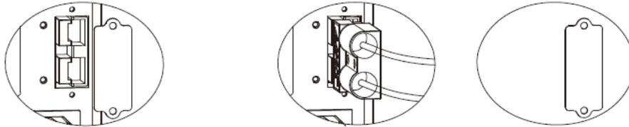
**Removecableretention clip. Plugin EBPcable. Retain the clip.**
