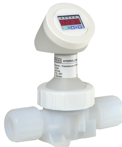
HYDRA-line Model HD, transducer 4 ... 20 mA, 2-wire system, with integrated digital display (HYDRA-Indicator) and in-line 1/2" flare process connection
