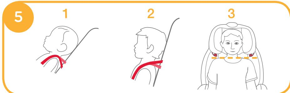
Squeeze the head support adjustment lever, meanwhile pull up or push down the head support until it snaps into one of the 10 positions.
