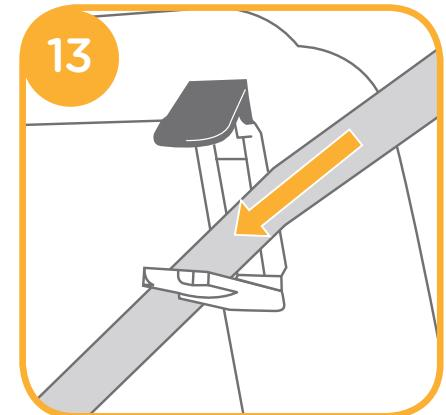
3. While pressing the child restraint, pull the belts to fasten the child restraint tightly and securely. 14
