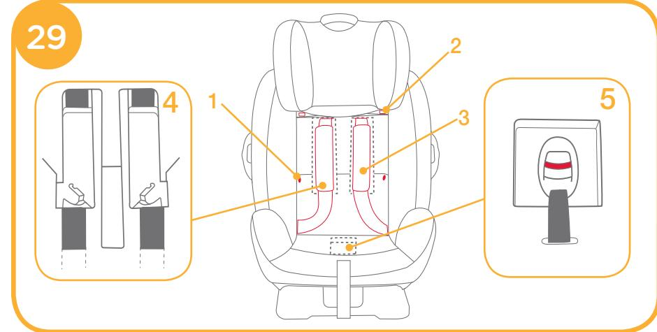
3. Detach the snaps and the hook and loop fasteners. 29 -1 & 29 -2
