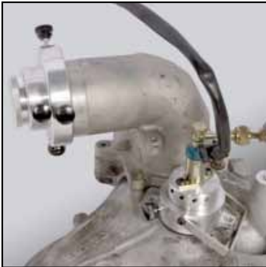
First, the EGR port is cleaned...
