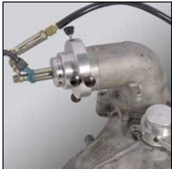
...then deposits are removed from the air intake manifold.
