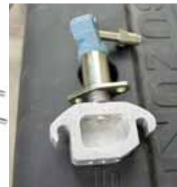
Specially designed Suzuki EGR adaptor
