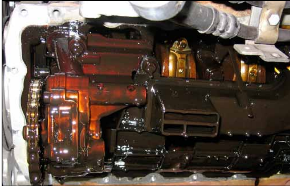
Sludged engine before service
