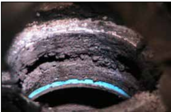
Deposit buildup in EGR assembly
