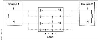
\* to power supply the product, make a strap between 103 (N) and 104 terminals (power supply input 104-106 on source ①).
