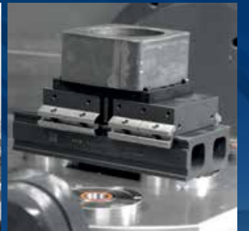
Clamping blank parts A wide range of grip jaws.
