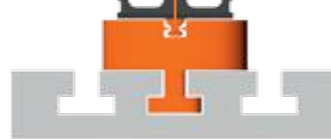
Clamping via the zero point clamping system (clamping pot).
