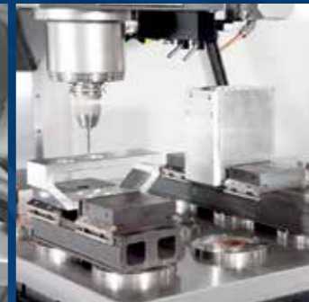
Clamping finished parts for instance using front pull-down jaws.
