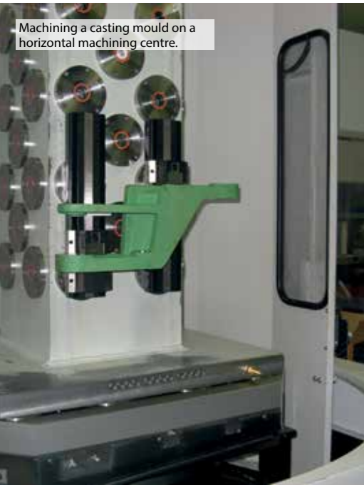
Clamping rail SL 120 1. Clamping with grip inserts.
