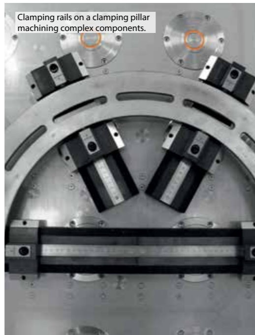
Workpiece clamping with a jig on a horizontal machining centre.
