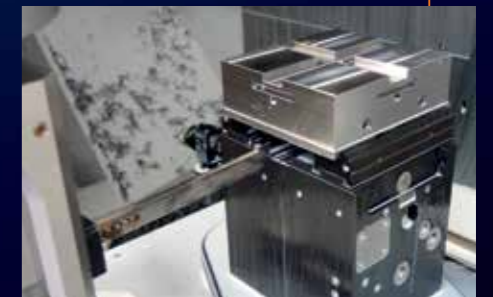
Blank parts are gripped directly and exchanged.
