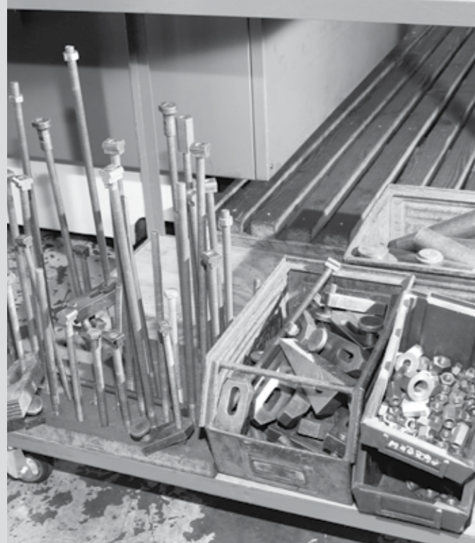
Unmanageable collection of mechanical clamping elements. Long and complicated clamping procedures and alignment of the component.
