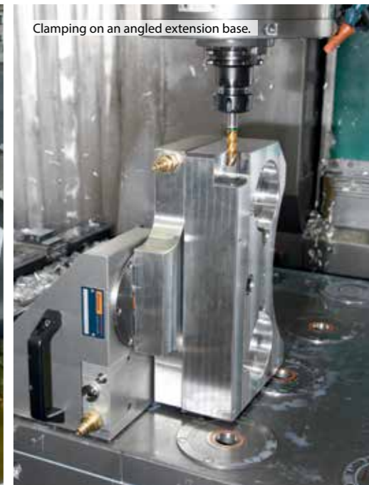
Manual clamping situation in combination with zero point clamping system (pillar).
