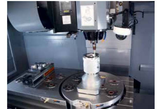
Side wing with NC vice, round table with 1-pot extension base and directly clamped component.
