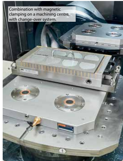
Jig adapter plate on the clamping pillar Machining on a horizontal machining centre without interference contours Reduces the set-up time by approx. 80%.
