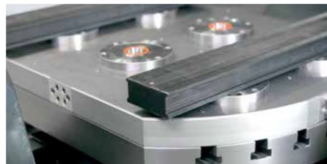
Clamping via the zero point clamping system (clamping pot).
