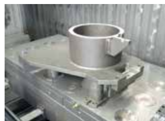
Flexible clamp on a GARANT ZeroClamp zero point clamping system
