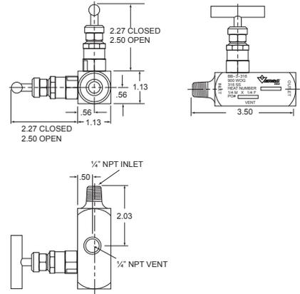
The Versa Block and Bleed valve is a traditional isolation valve. It consists of "block" and "vent" needle valves to isolate and vent downstream pressure during gauge changes.
