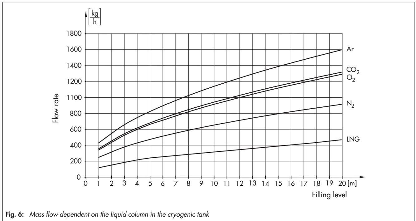
**Fig. 6:** Mass flow dependent on the liquid column in the cryogenic tank
