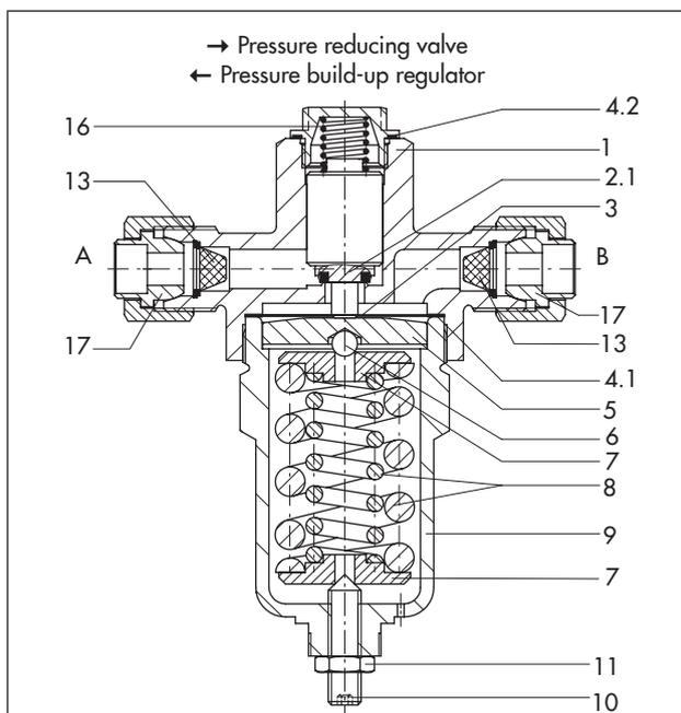
**Fig. 3:** Type 2357-1 Pressure Build-up Regulator or Pressure Reducing Valve (PN 50)
