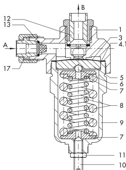
**Fig. 4:** Type 2357-2 Excess Pressure Valve (PN 50)
