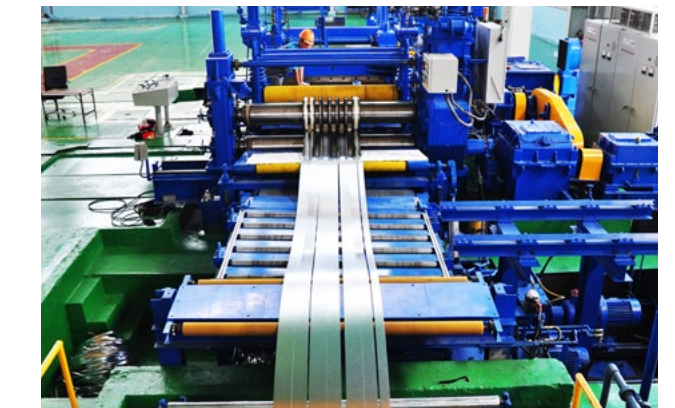
15. Kiểm tra/ Inspection of slitted steel
